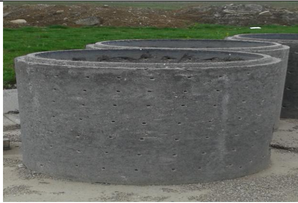
Camere aerisire gaz
